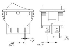
NOTE: Available with S1 & S2 mounting style and Q contact rating only. Shown in Pos. 1
